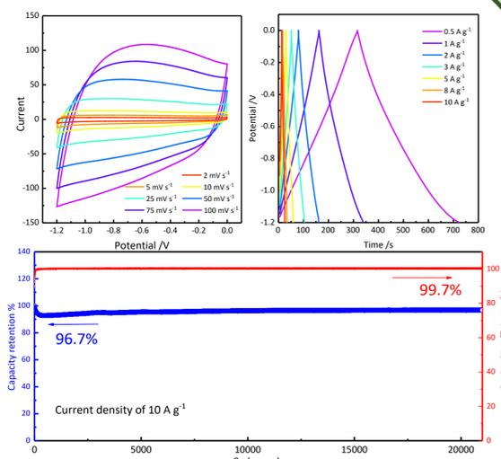
Electrochemical measurements: 6M KOH aqueous electrolyte in the potential range of -1.2 – 0 V vs. SCE in a three-electrode system.
