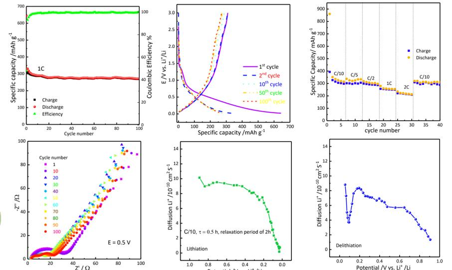
➤ 1 M LiPF<sub>6</sub> in EC: DMC as electrolyte, 0.01 V ≤ E ≤ 3.00 V, 1C = 300 mA g<sup>-1</sup>
