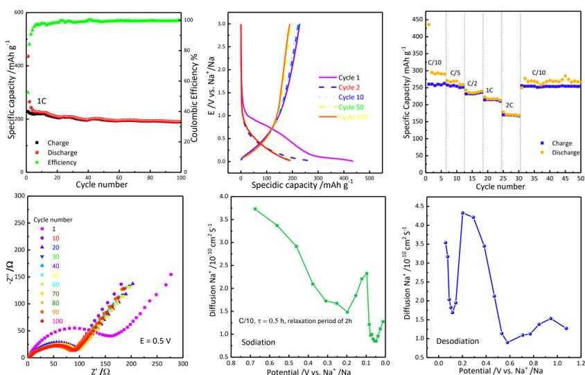
➤ 1 M NaClO<sub>4</sub> in EC: PC electrolyte, 0.01 V ≤ E ≤ 3.00 V, 1C = 300 mA g<sup>-1</sup>
